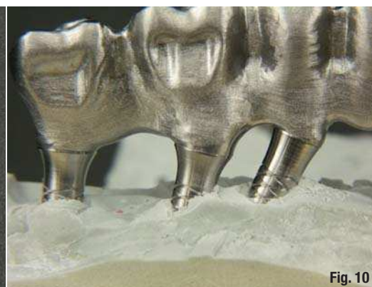
Figs. 9 & 10: Cr-Co framework machined before scraping and finishing.
